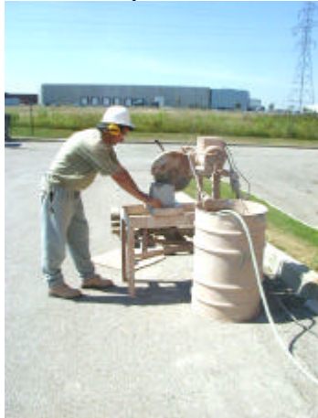
Figure 1: Little dust produced by wet cutting
