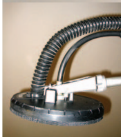
Figure 2. Shrouded ventilated rotary sander attached to vacuum.
