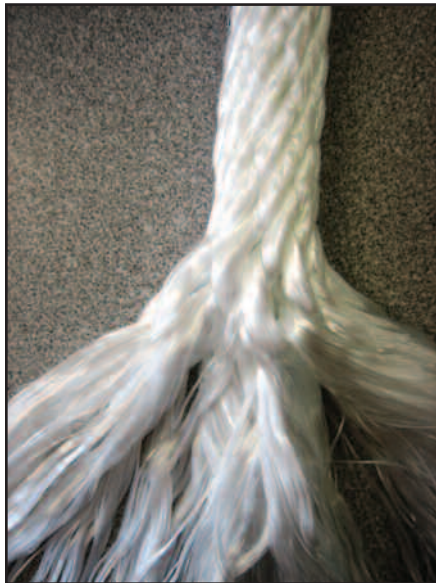
A solid braid rope is very flexible. It can stretch under load.
