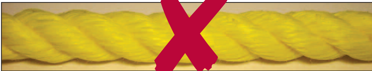
Do not use utility rope for lifelines.
