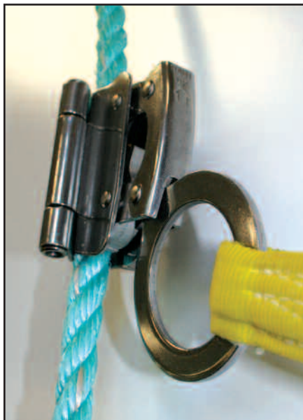
This three-strand twisted rope is made from a polypropylene/polyethylene blend. The different-coloured strand indicates that the material is a blend.
