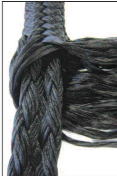
A double braid rope consists of a braided sheath covering a braided core. Both the core and sheath support the load, so they must be aligned. If the sheath bunches up, you decrease the rope's strength by 50%.
