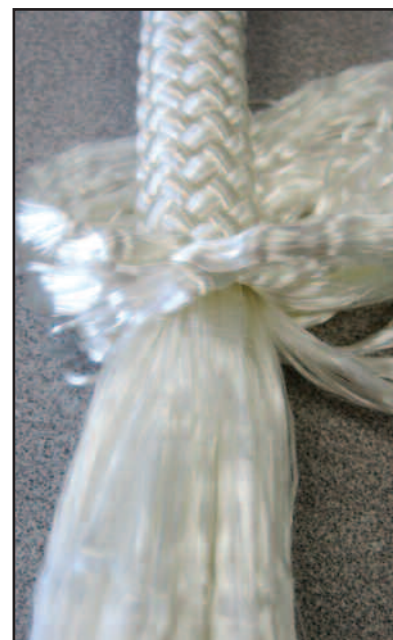
Kernmantle rope is very durable. The fibres in the core run straight. All of the rope's strength is in the core, while the braided sheath protects the core.
