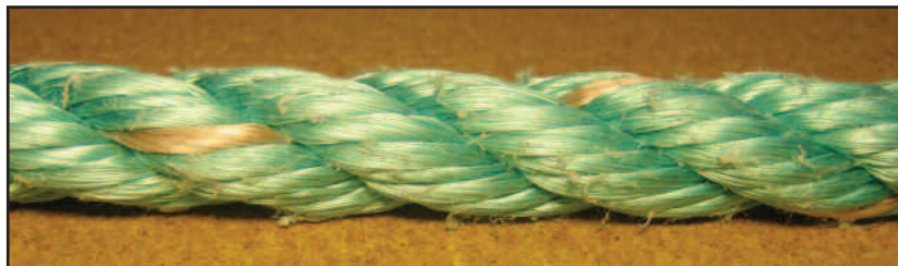
This three-strand twisted rope is made from a polypropylene/polyethylene blend. The different-coloured strand indicates that the material is a blend.
