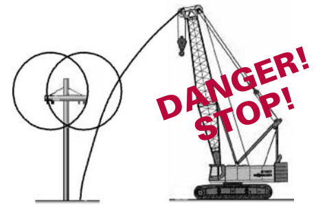
This crane boom could reach within the minimum distance.
