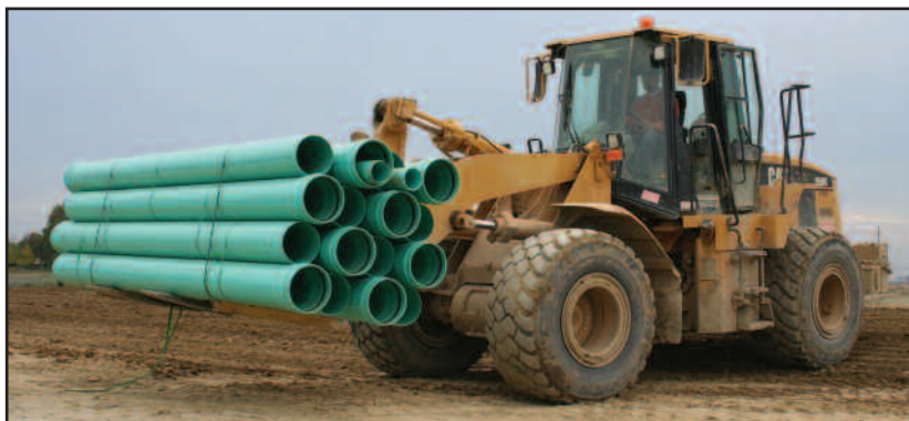
Stay clear of material being moved. You can be crushed by the material if it falls or comes loose.
